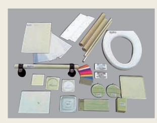
In order to solve this problem, Daicel Polymer Ltd. has developed CELBLEN, a reinforced plastic made with high-purity cellulose fiber. This fiber is refined from wood and bamboo sources and is almost completely decomposed when incinerated.\* Moreover, it increases the colorability and printability of plastics and is expected to find wide application in injection molding and the production of sheets, foamed products, and extrusions.
