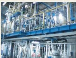
A pilot plant incorporating adipic acid manufacturing technology using NHPI catalyst. This plant is now under construction on the premises of the Himeji Research Center.
